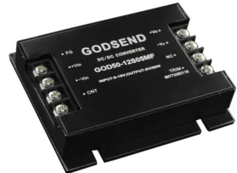
The industrial isolated DC-DC converter also features 83% conversion efficiency, 50W maximum output power, 0A to 10A output current range, and operates within -40°C to 85°C temperature range. This converter is used in portable power supply systems on the chassis, railway locomotives, new energy, communications, electric power, industrial control, and occasions where input and output are isolated.
