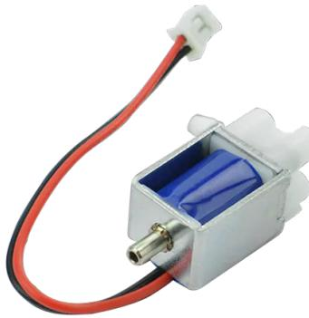
The DFR0866 6V 2-position 3-way air valve includes a Common interface (COM), a Normally Open interface (NO), and a Normally Closed interface (NC). The user can determine which interface is connected to the Common interface by powering the valve on and off.
