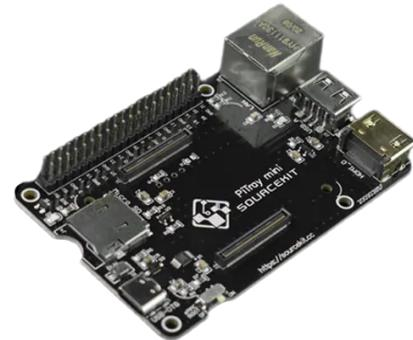
The PiTray mini offers boot switching for normal and programming modes and can fit in most of the same cases as the Raspberry Pi IO board. This PiTray mini features 5V input power and is available in 85mm x 56mm dimensions.
