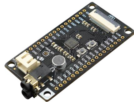
The FireBeetle Covers-Camera and Audio Media Board features 3.7VCC to 5.5VCC operating voltage, 3.3V output voltage, and a user-defined button. This board can be an MP3, a recorder, and a camera with any FireBeetle mainboards.
