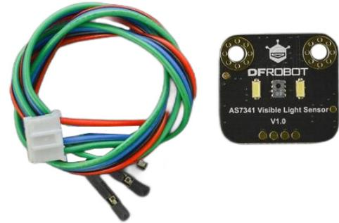
The AS7321 11-channel visible light sensors integrate a dedicated channel to detect ambient light flicker. These sensors come with six independent 16-bit ADC channels for data processing in parallel. The AS7321 11-channel visible light sensors are used in the applications such as high accuracy color detection and matching, color mixing effect detection, lighting color temperature adjustment, lighting atmosphere control, and modern plant cultivation.
