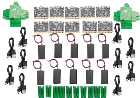
The micro:bit v2 club 10-pack features a Nordic nRF52833 processor, MEMS microphone, speaker, and capacitive touch sensor.
