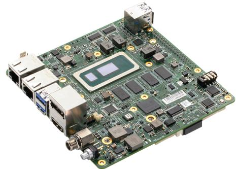
The UP Xtreme boards operate at 0°C to 60°C temperature range and feature 12V to 60V wide voltage power input, 2 RS232/422/485 10-pin headers, a built-in audio jack, and Time-Sensitive Networking (TSN) to facilitate communication in a connected factory. These boards offer flexible expandability with both a 40-pin and 100-pin connector, M.2 2230, M.2 2280 slots, and mPCIe slots.
