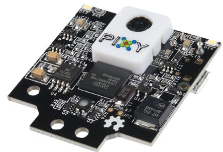
The SEN-14678 camera includes an NXP LPC4330 processor and the ON Semiconductor MT9M114 image sensor with 1296 x 976 resolution with an integrated image flow processor. This Pixy2 camera offers 264KB RAM, 2MB Flash, 20lumens integrated light source, and consumes 140mA typical power. The Pixy2 functions on a color-based filtering algorithm to detect objects as it is fast, efficient, and relatively robust.
