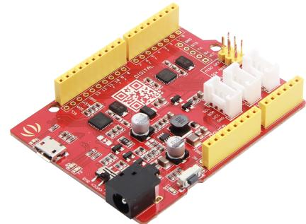
The V4.2 Arduino-compatible board can be programmed with a micro-USB cable, and powered with a 7 to 15VDC jack input. This V4.2 Arduino-compatible board features 14 digital input pins, 16 analog inputs, and 16 PWM outputs. Three on-board Grove interfaces allow for easy connection to Groves.
