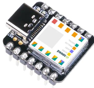
The XIAO pre-soldered board is compatible with Arduino IDE, breadboard-friendly, and includes power pads for the battery power supply. Typical applications include wearable devices, rapid prototyping, DIY keyboard, and USB development.
