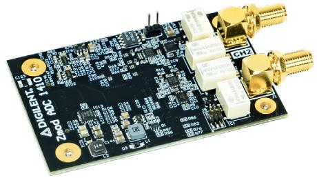
The Zmod module when coupled to a baseboard using SYZYGY expansion, such as the Eclypse Z7 or Genesys ZU, the combination becomes a powerful prototyping platform for instrumentation, and high-speed control, and SDR products. This module operates on an absolute resolution of 0.13mV for low range or 3.12mV for high range, an accuracy range of  $\pm 0.2\%$ , and a 100MS/s sample rate.
