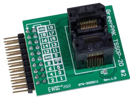
The SLG46827-A IC is designed into the TSSOP20 socket on the Socket Adapter, which then connects to the socket connector on the advanced development board. The advanced development board can then be connected to a PC running the GreenPAK designer software.
