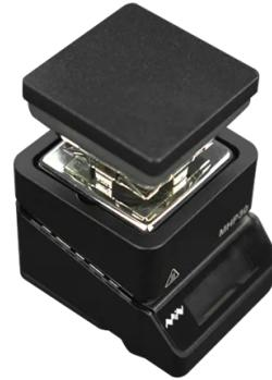
The MHP30 heating station is a portable tool with a square tower shape, a total height of only 5.2cm (2 inches), and a heating area of 3cm x 3cm. This compact preheater is highly-efficient and helps in preheating and desoldering applications. The MHP30 includes a LED screen that displays the current temperature of the heating element in real time to better control the heating temperature.
