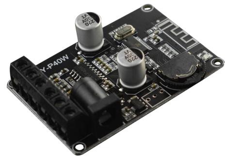
The DFR0675-EN board includes power supply reverse connection protection, and short circuit protection. This amplifier board can be operated with a Bluetooth 5.0 remote control, up to 15 meters of communication distance. The DFR0675-EN board works in an operating voltage range of 5V to 24V.
