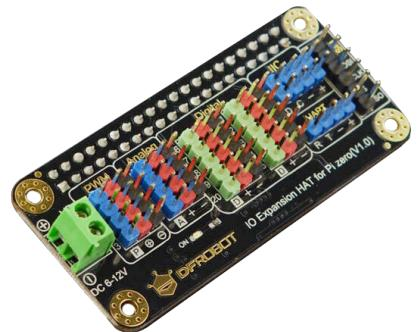
The PWM and analog ports that lead out through the onboard MCU STM32 can communicate with Raspberry Pi via I<sup>2</sup>C. This expansion board supports a 5V power supply and 3.3V sensor modules, its PWM port can be powered by external power (6V to 12V) or Raspberry Pi (5V). The IO expansion HAT is compact and can be conveniently used in Raspberry Pi to control PWM output or read ADC input.
