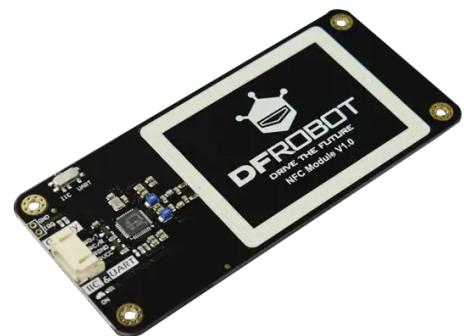
This Gravity module exhibits the ability to effortlessly read and write various NFC cards using a USB to UART converter and PN532 compatible PC software through UART. This module is used in various 3.3V/5V controllers such as Arduino, micro:bit, FireBeetle ESP32, and FireBeetle ESP8266 when using the I<sup>2</sup>C interface.
