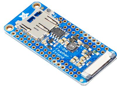
The user can create a frame buffer using CircuitPython or Arduino libraries and write that to the display with desired pixels. The eInk Feather Friend is designed with a 256Kilobit (32Kilobyte) SRAM chip and shares the SPI port hence needing just one extra pin. The user can control up to a 4.2" 300x400 tri-color display (300x400 x 2 colors/8 bits-per-byte = 30KB).
