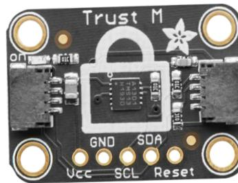
This chip can store private keys securely, as well as generate true random numbers. The board comes with a bit of 0.1" standard header in case the user wants to use it with a breadboard or perfboard. The breakout board features four 2.5mm (0.1") mounting holes for easy attachment. This breakout board is RoHS2 compliant.
