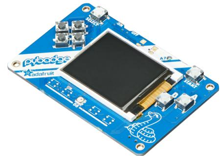
The 462x PyBadge starter kits also feature the same processor chip, QSPI flash, on/off switch, buttons, buzzer, light sensor, battery circuit, and one NeoPixels in the center front. The low-cost version is available with pared-down hardware and does not have Feather headers, JST STEMMA connectors, LIS3DH accelerometer, or optional speaker connection.
