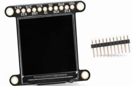
The LCD display is ideal for smartwatches and small electronic devices but always by MIPI interface. This SPI display features a friendly display driver and works with any and all microcontrollers or microcomputers. This display is RoHS2 compliant.
