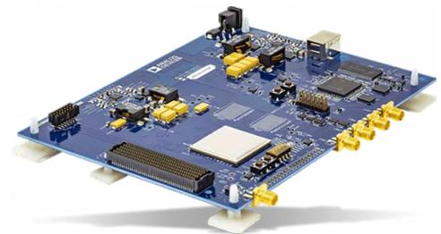
Additional equipment needed includes an Analog Devices high speed ADC evaluation board, a signal source, and a clock source. Once the kit is connected and powered, the evaluation is enabled instantly on the PC. The ADC capture board enables numerous expansion and evaluation possibilities by virtue of its powerful reconfigurable FPGA core.
