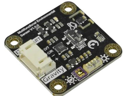
The environmental sensor features an onboard MCU processing chip that converts raw sensor data into values with the standard unit for direct use. This multifunctional sensor supports two communication methods (UART and I<sup>2</sup>C). The multifunctional Gravity sensor provides two versions: Gravity and Fermion (breakout), and complete Arduino and Python libraries. Typical applications include indoor and outdoor environment detection systems and environmental monitoring work.
