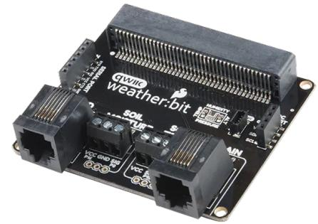
The weather:bit connects to the micro:bit via an edge connector at the top of the board, making setup easy. This creates a handy way to swap out micro:bits for programming, while still providing reliable connections to all of the different pins on the micro:bit. This board also includes serial and I<sup>2</sup>C headers on the weather:bit for optimized connectivity if you so choose.
