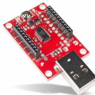
The dongle offers a reset button, a voltage regulator for power supply, and four LEDs (RX, TX, RSSI, and power indicator) to help debug the XBee. This XBee Explorer dongle breaks out each of the XBee's I/O pins to a pair of breadboard-compatible headers.
