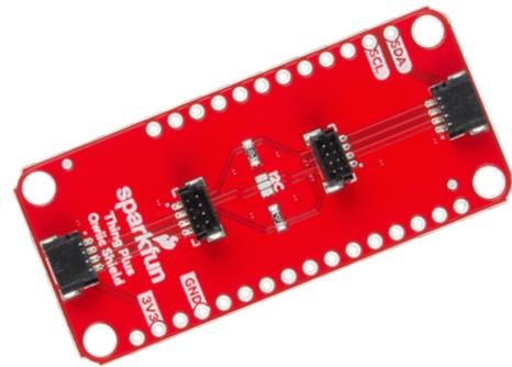
The Qwiic Shield for Thing Plus comes with one 12-pin and one 16-pin headers. You will need to solder the headers to the shield and, if necessary, to your Thing Plus or Feather board. Take care to match the markings on the Qwiic Shield to the appropriate pins on your Thing to avoid possibly damaging your boards.
