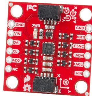
The ICM-20948 features 3-axis gyroscope, 3-axis accelerometer, 3-axis compass, and digital motion processor that offloads the computation of motion processing algorithms from the host processor, improving system power performance.
