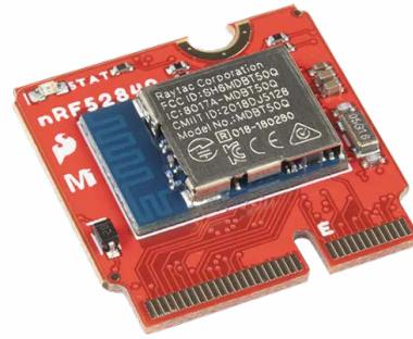
The MicroMod nRF52840 processor board features the same Raytac MDBT50Q-P1M found on the Pro nRF52840 Mini. This module includes an integrated trace antenna, fits the IC to an FCC-approved footprint. It also includes decoupling and timing mechanisms that would need to be designed into a circuit using the bare nRF52840 IC.
