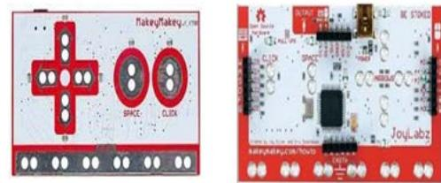
The makey makey classic is a two-sided circuit board comes with a top side and back side. This kit features 6 inputs on the front of the board that can be attached to via alligator clipping, soldering to the pads, or any other method. The kit also features 12 inputs on the back, 6 for keyboard keys, and 6 for mouse motion which can access with jumpers via the female headers.
