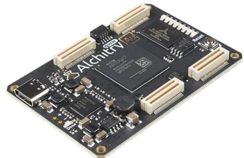
The DEV-17514 Alchitry Au+ Development Board is powered by 5V through USB-C port, 0.1" holes, or headers. This Au+ board also offers a 100MHz on-board clock, a USB-C connector to configure and power the board, and a USB to serial interface for data transfer. The DEV-17514 Alchitry Au+ development board is RoHS compliant.
