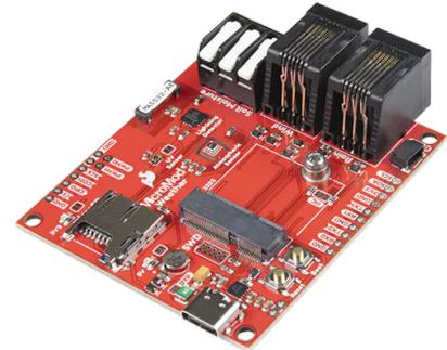
This board also features a 3-pin latch terminal to add an external soil moisture sensor as well as a pair RJ11 jacks to plug in the wind and rain sensors included with Weather Meter Kit. The weather carrier board offers a MicroSD card slot so users can plug in an SD card to log all of that glorious weather data using the MicroMod processor of user's choice.
