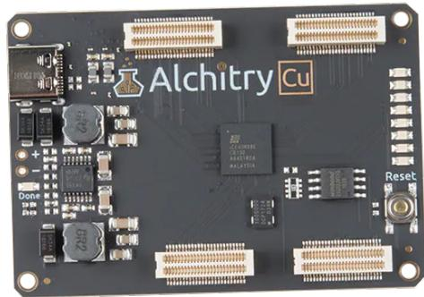
The Cu possesses 79 I/O pins with eight general-purpose LEDs, a 100MHz onboard clock that can be manipulated internally by the FPGA, a USB-C connector to configure and power the board, and a USB-to-serial interface for data transfer. The Alchitry Cu is also able to expand its own hardware capabilities by adding prototyping spaces, buttons, LEDs, and more.
