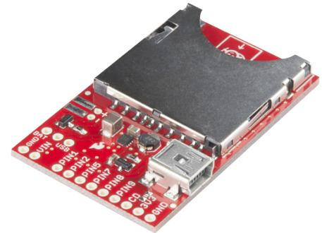
To use the mini-USB or battery inputs for power, it must populate the 3-pin jumper and set it to either 'BAT' or 'USB.' Another way is to power the board using Vin and GND without the use of a jumper.
