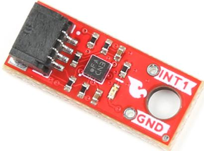
The Bosch Sensortech<sup>®</sup> BMA400 sensor offers a full-scale acceleration range of  $\pm 2g/\pm 4g/\pm 8g/\pm 16g$  with ultra-low current consumption of  $<14.5\mu A$  while operating at its peak performance settings. This sensor also includes a complete feature set for on-chip interrupts, including auto wakeup/low power, step counter, activity recognition, orientation detection, and tap/double taps.
