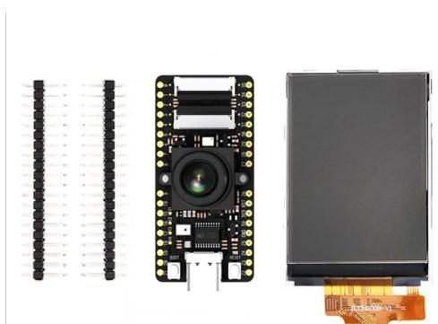
The Sipeed MAIX bit suit with LCD, camera comes with accelerators and peripherals like AES accelerator, SHA256 accelerator, FFT accelerator, OTP, UART, WDT, IIC, SPI, I<sup>2</sup>S, TIMER, RTC, and PWM. The MAIX features a model compiler to compile models to its own model format and a RISC-V dual core 64bit CPU and a high-speed UART and JTAG interface for debugging.
