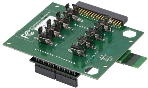
The JN5169XK010 expansion kit is used to create a node that provides switch, level control, and LED functionality.
