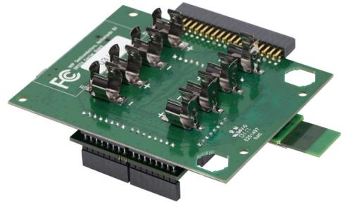
The JN5169XK010 expansion kit is used to create a node that provides switch, level control, and LED functionality.
