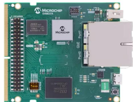
This evaluation board features a LAN9662 AVB/TSN switch, an internal real-time engine, and a 600MHz Arm® Cortex® A7 CPU. The EVB-LAN9662 board offers two tri-speed (10/100/1000M) RJ45 front ports using internal copper PHYs. This board supports a USB 2.0 host port, a micro-USB 2.0 console port, a reset status LED, and per-network port status LEDs. The EVB-LAN9662 board is powered by the micro-USB port, the edge connector, or the expansion header.
