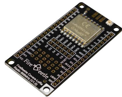
This module provides a maximum transmission rate of up to 300Kbps. The TEL0125 module supports long-range monitor, FSK modulation, and provides a maximum transmission of 37.5Kbps. This module is widely used in remote home automation detection, wearable device, and health monitoring.
