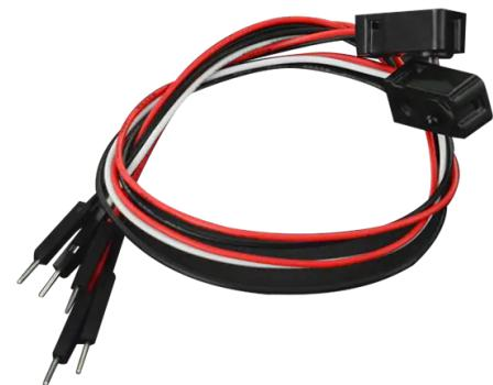
The SEN0503 sensor works by having an emitter that sends out a beam of human-invisible IR light, then a receiver across the way that is sensitive to that same light. When something passes between the two and is not transparent to IR, the beam is broken, and the receiver will output a signal to let the user know. In smart robot competitions, this IR sensor can be used with Arduino for simple motion detection, speed detection, and timing.
