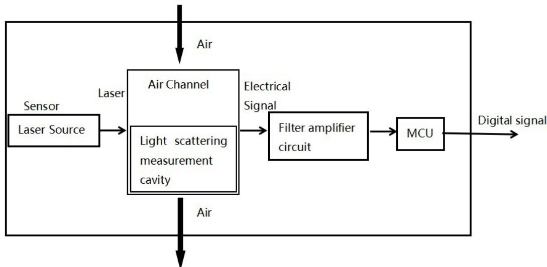
The SEN0460 sensor adopts the principle of laser scattering, to make the laser irradiate the suspended particles in the air to produce scattering. At the same time collect the scattered light at a certain angle and obtain the curve of the intensity of the scattered light with time.
