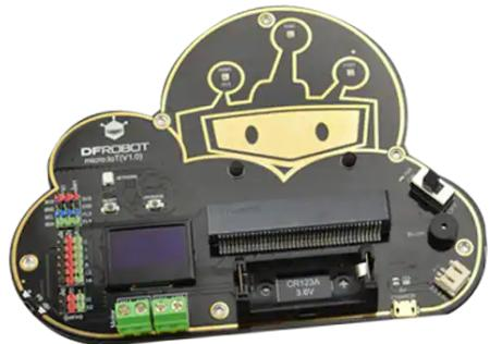
The micro: IoT board comes in a cloud-based design that is more suitable for the IoT theme. This IoT development board runs on a 3.6V CR123A lithium rechargeable battery and offers small size, high capacity, and high safety. The micro: IoT development board employs an easy interface and does not need complicated background knowledge to build IoT applications.
