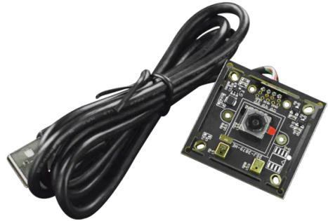
This camera module comes with a digital microphone that captures the sound of 5 meters around the camera while recording the video. The USB port design makes it easier to use with a Raspberry Pi and Jetson Nano mainboard. The USB camera can be embedded into various devices and is perfect for high-quality video systems, biometrics recognition, industrial photography, and HD monitoring.
