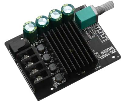
This Bluetooth board has four quality 470uF capacitors that produce stable output; The board also comes with a heat sink and adopts an excellent power module, allowing it to work steadily under a long time of high output. Apart from that, the board includes bottom/top protective panels and supports auto overheat protection and auto short circuit protection.
