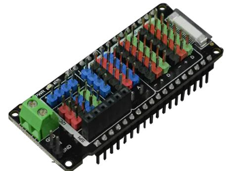
The Gravity IO shield allows a convenient connection between DFRobot Gravity sensors and FireBeetle 2 series. No soldering is required. This expansion board is specifically designed for FireBeetle 2 controllers' series: M0, ESP32-E, and is unsuitable for the original FireBeetle Series.
