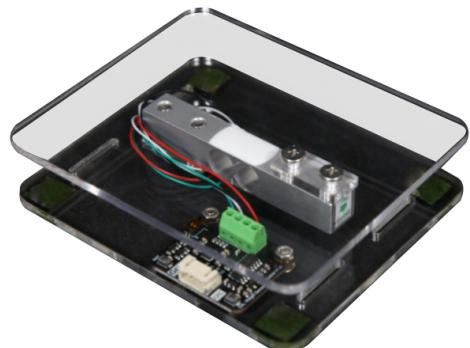
The HX711 I<sup>2</sup>C weight sensor kit is compatible with the Arduino series, micro:bit, ESP32, and Raspberry Pi and features a built-in signal adapter board. This kit offers a 1g to 1000g measuring range and operates at a 3.3V/5V range. Typical applications include a simple electronic scale, daily necessities weighing, daily necessities remaining alarm, and IoT weighing platforms.
