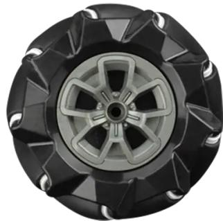
The FIT0767 black mecanum wheel offers low noise that allows the wheel to move stably and flexibly during operation. This mecanum wheel has a diameter of 97mm and is composed of 9 small rollers. These rollers are made of plastic and coated with quality and high-friction silicone rubber that are rugged and impact-resistant.
