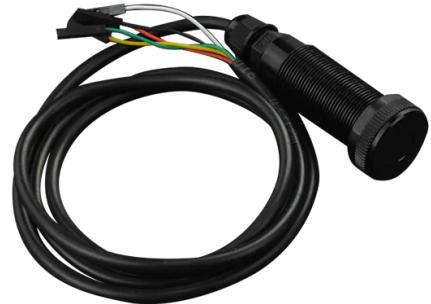
The DFRobot SEN0491 uses an invisible laser, and there is a voltage regulator circuit inside the module. By featuring a stable performance and UART output, the sensor has an alarm output line that will be triggered to output low steadily when the measurement distance is smaller than the user-set threshold.
