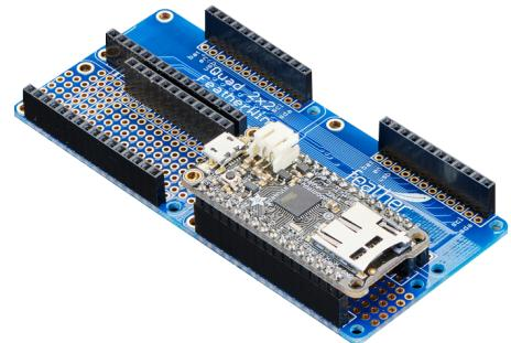
The Quad features three breakouts for each pin on a Feather and a bunch of plain grid proto holes. The four sets of pins are cross connected and there's a full strip of connected pads for GND and 3.3V. The Female headers will have to be soldered on to the PCB.
