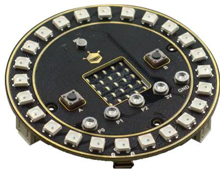
This micro: circular LED expansion board also supports PH2.0 interface power supply and the battery box or lithium battery power supply. The micro: circular LED expansion board features a MakeCode graphical programming and ultra-thin volume that is more suitable for wearable and strap applications.
