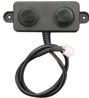
The A02YYUW communicates with the upper-host or other MCU with a 9600bit/s band rate that greatly shortens the developing cycles. Applications include backing car annunciator, obstacle avoidance robot, and object approach detection.
